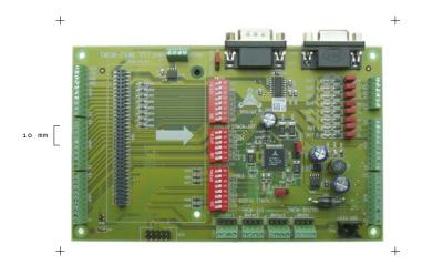
INFO The TMCM-EVAL is a baseboard which allows to evaluate the operation of the TMCM-Modules. All interface signals of the respective are available on screw terminal connectors. The inputs can be switched and the outputs are seen via LEDs. An integrated stepper motor driver TMC236 allows the operation of a 2 phase stepper motor when using the TMCM-100 or to the TMCM-301.
