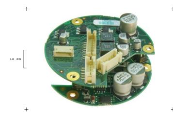
1-Axis Motor Mounted BLDC Servo Controller / Driver with Encoder Inf. 10A / 48V
