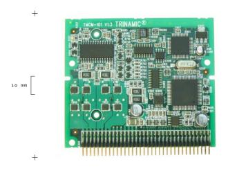
1-Axis Controller / Driver 3A / 28.5V with Encoder Inf.
