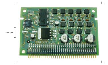
1-Axis Step / Direction or SPI Driver 3.5A / 48V
