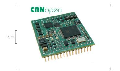
1-Axis Controller / Driver 2.0A / 28.5V with Encoder Inf.
