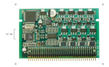
1-Axis Piezo Motor Driver 3kHz / 48V
