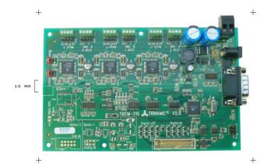
3-Axis Controller / Driver 1.1A / 34V
