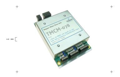
1-Axis Step / Direction Driver 7A / 75V
