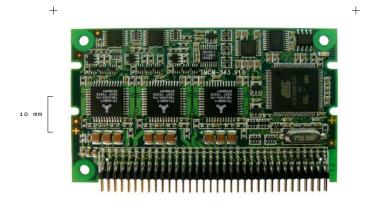
3-Axis Controller / Driver 1.1A / 34V
