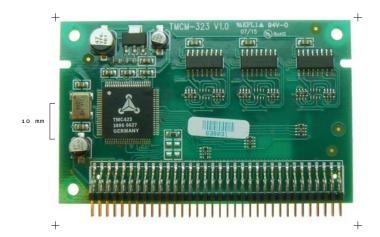
3-Axis Encoder Interface with SPI
