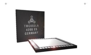
Three Phase Motor Driver with BLDC Back EMF Commutation hallFX™ and Current Sensing
