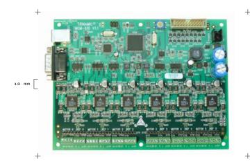
6-Axis Controller / Driver 1.1A / 34V
