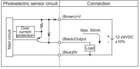
**%1: Load connection for NPN output X2**: Load connection for PNP output
